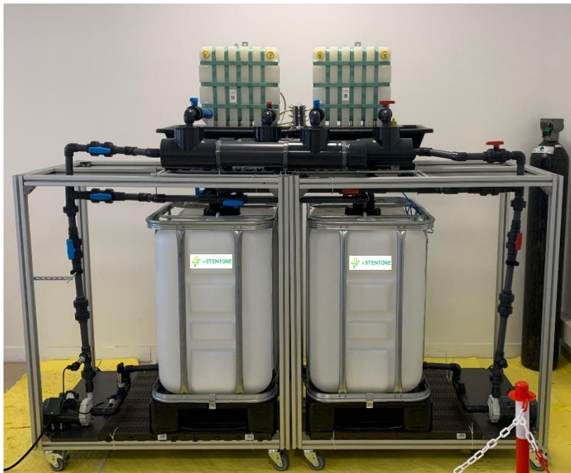
FIGURE 14: VRFB LAB-SCALE PROTOTYPE 4KW/8KWH
