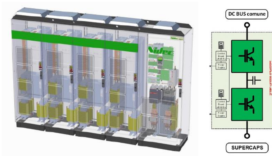
FIGURE 49: CAD REPRESENTATION AND CONCEPTUAL SCHEME OF THE DCDC CONVERTER DESIGNED TO INTERFACE THE NEW LTO SYSTEM WITH THE UFCS
